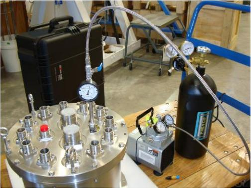
**\*\*CAUTION! INTERNAL PRESSURE INSIDE AN ENCLOSURE CAUSES TREMENDOUS FORCES THAT CAN CAUSE DAMAGE OR INJURY... MAKE SURE ENDCAP CLOSURE IS PROPERLY INSTALLED AND TIGHT, DO NOT EXCEED 10PSI INTERNAL PRESSURE, PLACE ENCLOSURE IN A SAFE PLACE AND STAND AWAY FROM ENDS IN CASE OF RELEASE**
