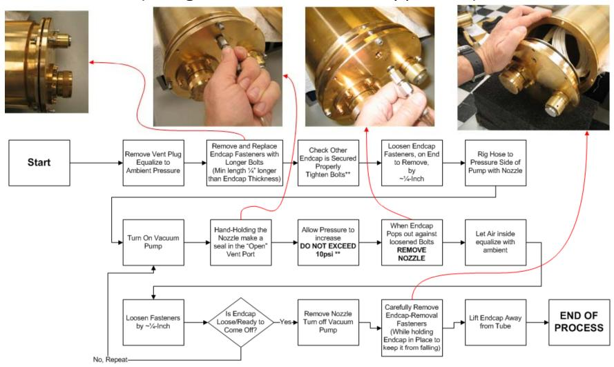
\*\*CAUTION! INTERNAL PRESSURE INSIDE AN ENCLOSURE CAUSES TREMENDOUS FORCES THAT CAN CAUSE DAMAGE OR INJURY... MAKE SURE ENDCAP CLOSURE IS PROPERLY INSTALLED AND TIGHT, DO NOT EXCEED 10PSI INTERNAL PRESSURE, PLACE ENCLOSURE IN A SAFE PLACE AND STAND AWAY FROM ENDS IN CASE OF RELEASE
