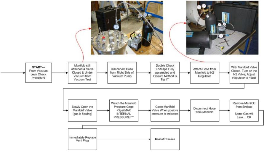
\*\*CAUTION! INTERNAL PRESSURE INSIDE AN ENCLOSURE CAUSES TREMENDOUS FORCES THAT CAN CAUSE DAMAGE OR INJURY... MAKE SURE ENDCAP CLOSURE IS PROPERLY INSTALLED AND TIGHT, DO NOT EXCEED 10PSI INTERNAL PRESSURE, PLACE ENCLOSURE IN A SAFE PLACE AND STAND AWAY FROM ENDS IN CASE OF RELEASE
