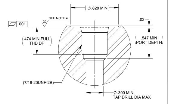
**DETAIL B - MOUNTING INTERFACE** STANDARD SAE #4 PORT PER SAE J1926 **MODIFIED AS NOTED ABOVE USE PARKER TOOL #Y34732**
