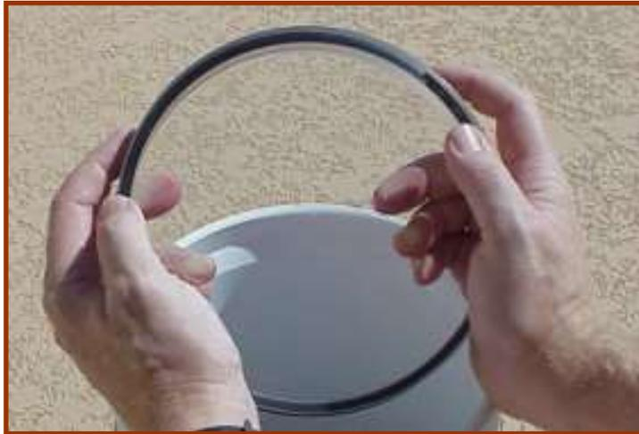
Stretch the o-ring by simultaneously applying inward radial pressure and circumferential translation until the seal buckles as shown.
