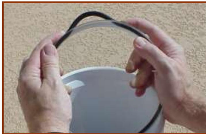
Grasp the buckled portion of the seal and remove the entire seal from the groove.
